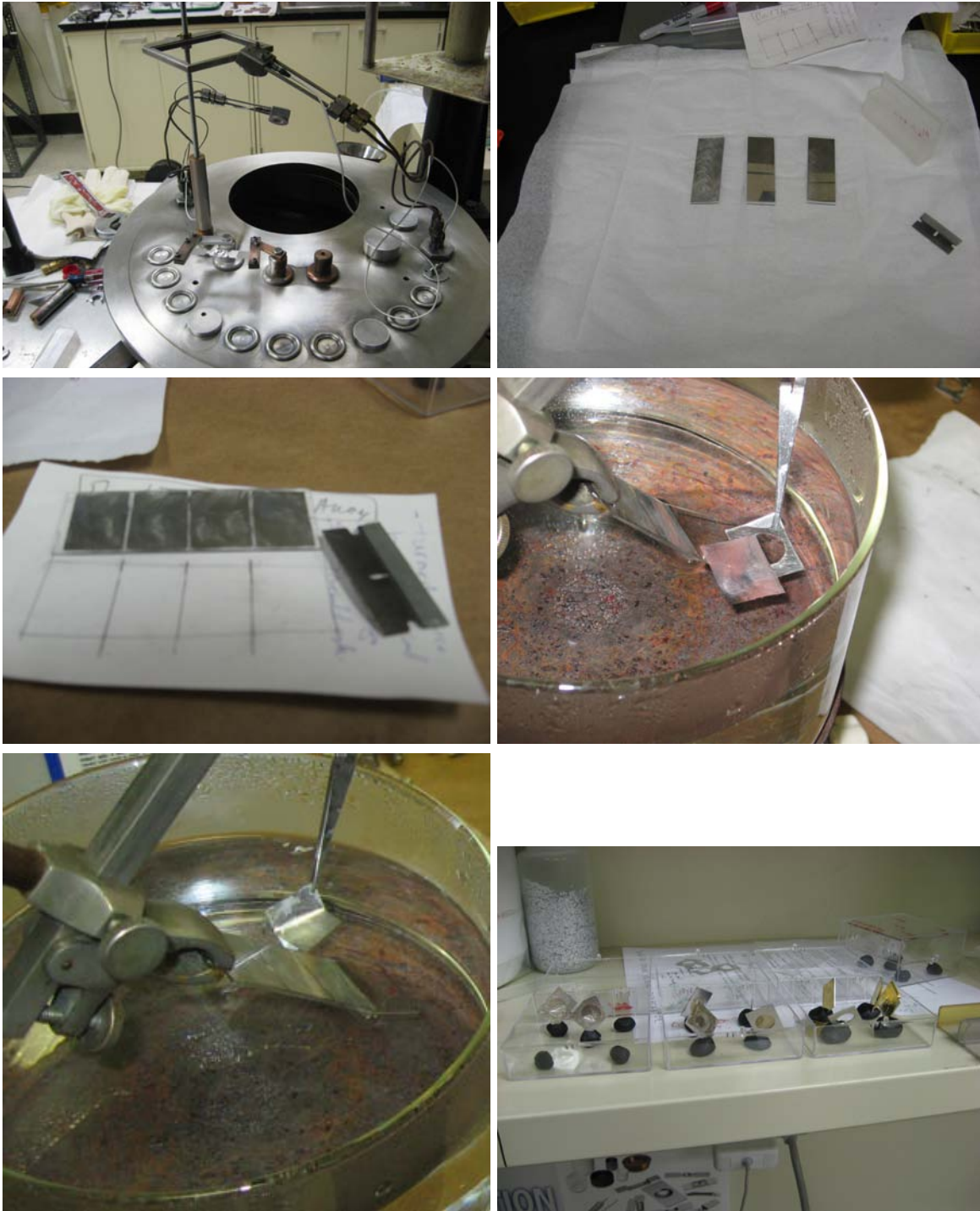
Figure 2.3: The target making process from beginning to end. In order from left to right and top to bottom: 1: The evaporator interior. 2: Slides newly coated with aluminum. 3: Properly scraped slides ready for floating. 4: Floating. 5: Mounting on the target holder. 6: The finished product (aluminum, gold, and carbon shown)
