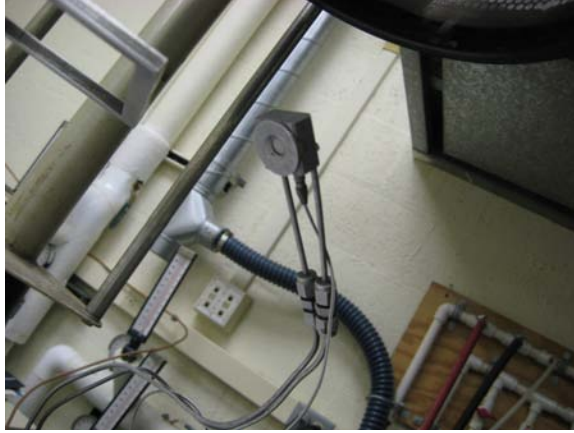
Figure 2.1: One of the two quartz crystal monitors used in our evaporator.
