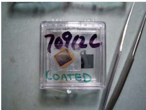
Fig 1.1 (Left) A (Ga,Mn)As sample that has undergone chemical wet etching and a coating process. (Right) A (Ga,Mn)As sample as grown.
