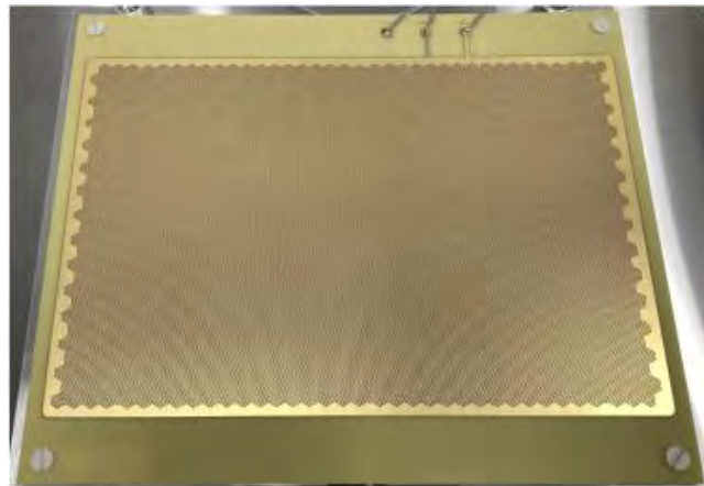
Figure 1. Multilayer-Thick Gas Electron Multiplier (M-THGEM) installed in the ND-Cube
