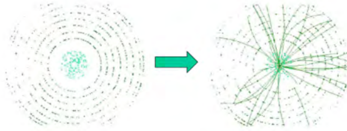
Figure 5: An illustration of the detector hits being converted to tracks [5].
