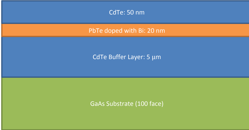
Figure 1: Diagram of sample structure. All samples were grown on a Gallium Arsenide wafer (100 face), followed by a Cadmium Telluride buffer layer 5 microns thick, then the Lead Telluride quantum well doped with Bismuth (20 nm), and finally a 50 nm layer of Cadmium Telluride.
