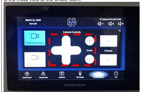
Utilize camera controls to adjust the view of the front (north wall) camera. If desired, the press and hold down the "Presets 2" button from more than 10 seconds so as to make this view the "Preset 2" view.
