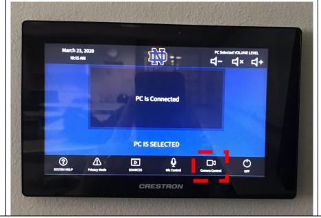
Crestron touchscreen = Camera Control button. Since, in Zoom, you are currently using/viewing the front camera, press the "Front Camera" button. Then utilize the center arrow keys and the Zoom +/- keys to adjust the camera to the desired view. Once the desired view is set, you can press and hold down the "Presets 2" button for 10 seconds or more so that this view is saved as the preset 2 view. Preset 1 is the initial view of the whole room.
