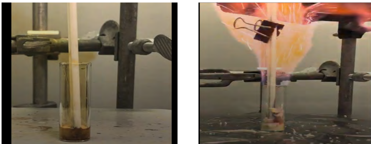
(a) Gas release of samarium oxide with ethanol as a solvent (b) Full combustion of samarium oxide with 2-methoxyethanol as a solvent
