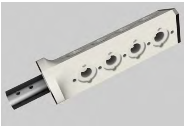
Figure 6: Stainless steel sample holder model. The center is dyed white where ceramic is in the current design.
