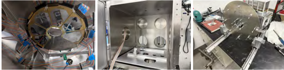
Figure 3: (a) Detector mount with Si Detectors (b) Target Chamber (c) Detector mount without detectors
