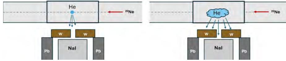
Figure 3: Gamma rays blocked by the tungsten shielding with point-like gas target (left) compared with extended gas target (right).
