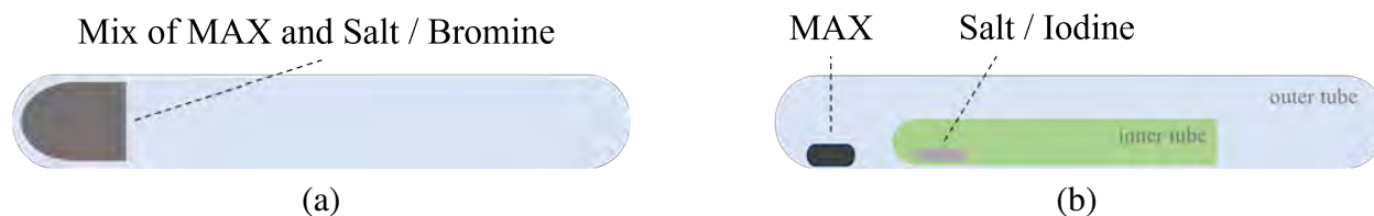
Figure 1: (a): MAX phase powder and halogen source loaded together in a single tube, used for direct \text{Br}_2 gas-phase and \text{FeCl}_3 molten salt etching. (b): MAX phase powder in the outer tube and halogen source in a semi-open inner tube, used for \text{I}_2 direct etching and in-situ gas-generation etching with \text{CuBr}_2 , \text{FeCl}_3 , and \text{FeBr}_3 .
